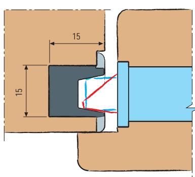
**Easy-matic application on flush doors with Mediana Polaris lock**
