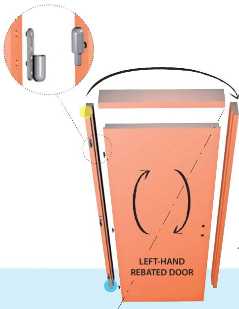
**In the manufacturer's premises** the male part of the hinge is fastened to the door panel, while the frame is pre-drilled. The female part can be affixed once the hand of the door is decided.
