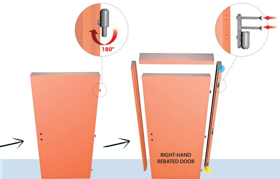
**In the building site**, it just takes the rotation of the hinge body of 180° in order to change the hand of the door.
