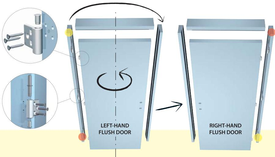
**In the building site** Twin is assembled and installed once the hand of the door is decided. Throughout the installation process, the oval holes allow an accurate vertical adjustment of the door leaf. At the end of the operations the third screw fastens the hinge.
