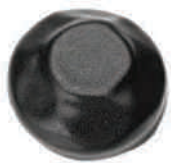
Clavo 10 Clavo forjado 10 Clavo redondo de 10 mm. Nail 10 10 Wrought iron nail Round 10 mm. nail
