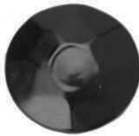
Clavo 20 Clavo forjado 20 Clavo redondo de 20 mm. Nail 20 20 Wrought iron nail Round 20 mm. nail
