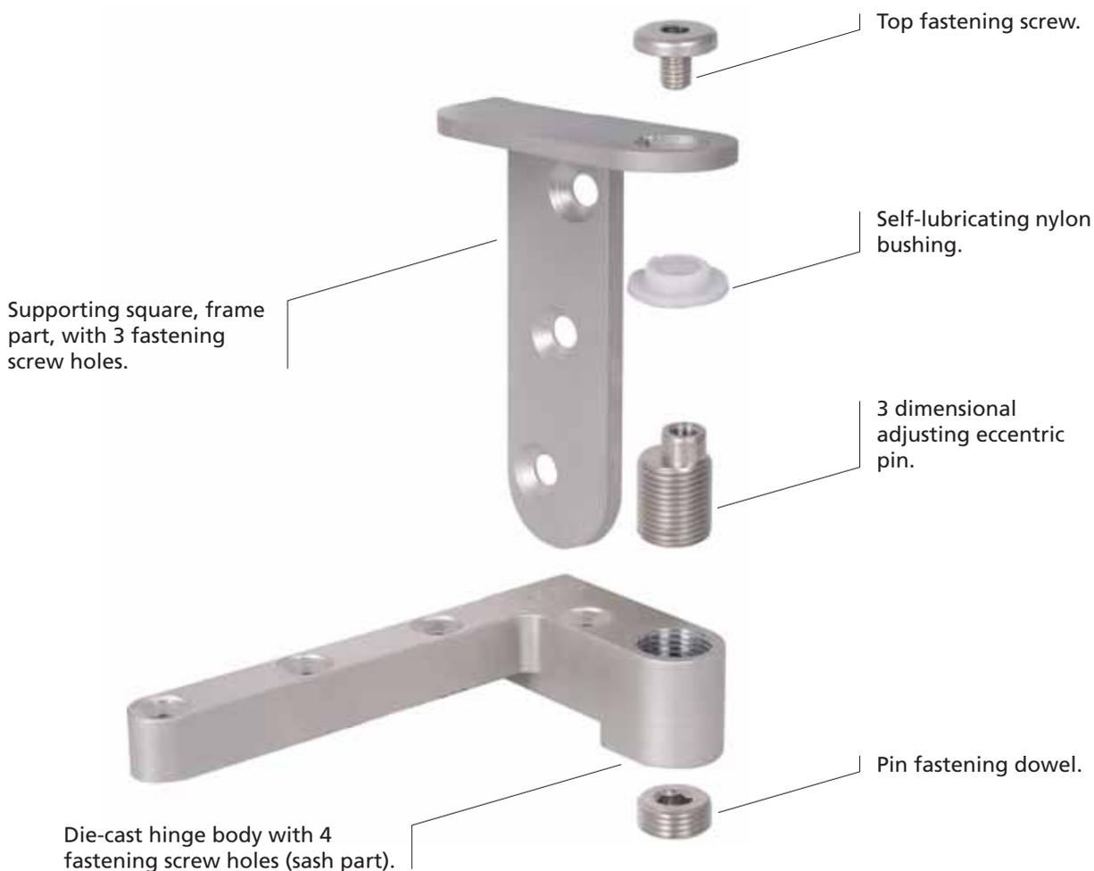
The eccentric pin allows the adjustment on 3 dimensions when door is installed.
